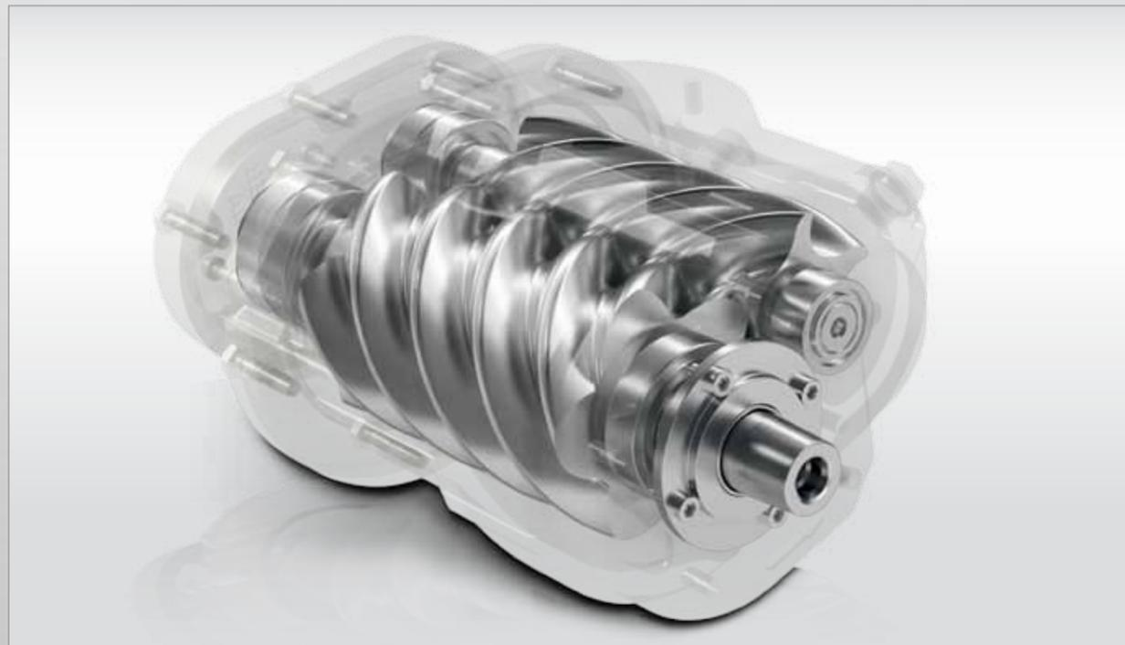
Schraubenkompressorblock mit dem energiesparenden SIGMA PROFIL
