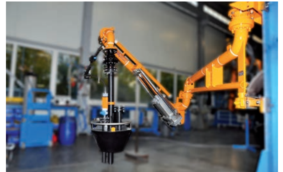
Loading arm with interior lining, DN 80/50, pneumatic lifting/lowering, counterbalancing using gas springs
