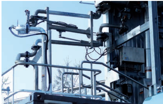
Top double loading arm, fully hydraulic, stainless steel
