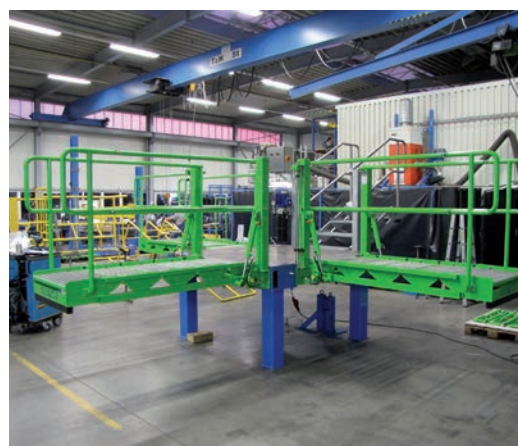
Folding stairs, hydraulic, with special acid-resistant paint and GRP steps
