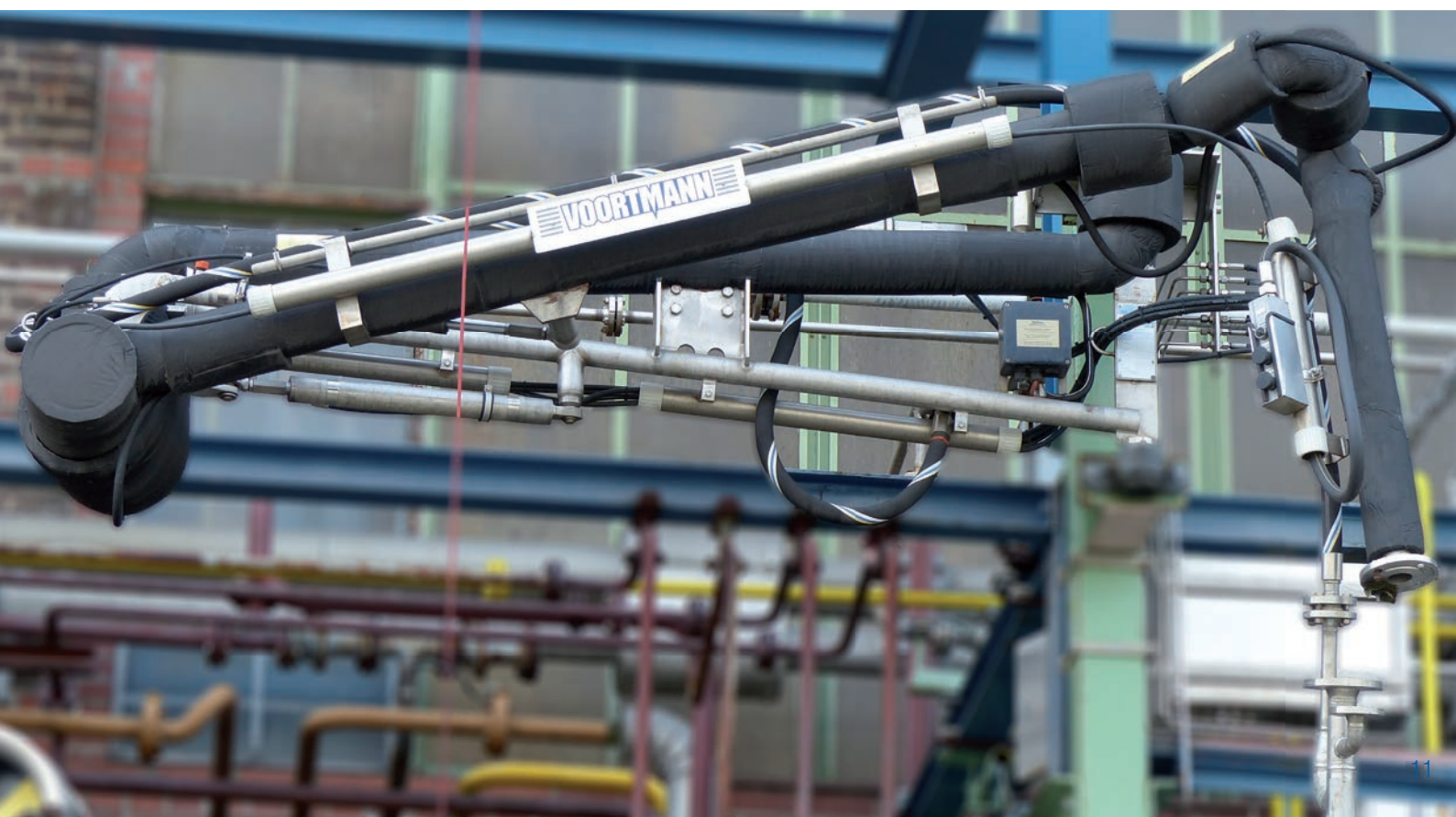
Loading arm, insulated and electrically heated
