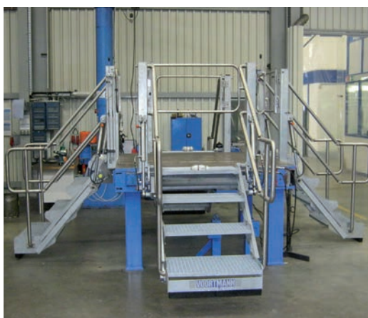
Folding stairs, hydraulic, with manual lever valve
